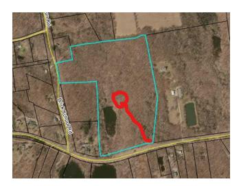
The proposed gravel surface driveway will be approximately 650' in length and graded and bermed to drain into proposed stormwater infiltration areas along the side of the driveway in regulated area.
