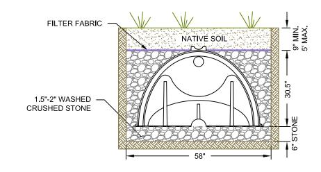
**CULTEC RECHARGER 330 SYSTEM** TYPICAL CROSS SECTION DETAIL
